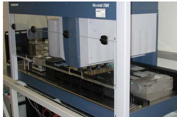
Fig 1: Preparation of the 35k Chip using a Hamilton Workstation
