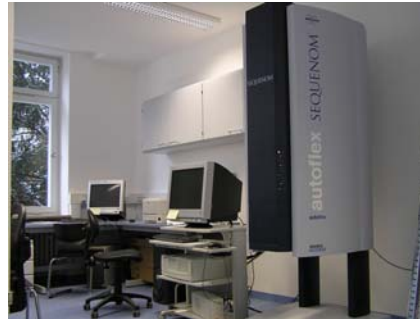
Fig 1: MALDI-TOF based high throughput genotyping system Autoflex (Sequenom; San Diego, USA) at the TU-Munich.
