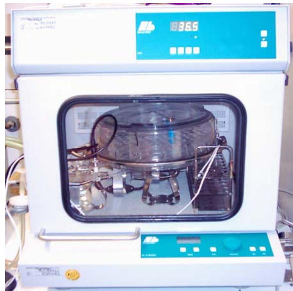
Fig 1: Hypoxia chamber. The temperature-controlled incubation chamber allows continuous monitoring of the atmosphere inside the chamber and the cell culture medium, especially the oxygen partial pressure.
