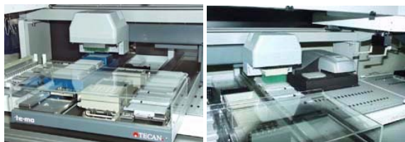
Fig 3 (left): Tecan te-mo with a high precision head and cooling unit for MTPs. (right): Tecan te-mo with standard head and PW384 for washing MTPs.
