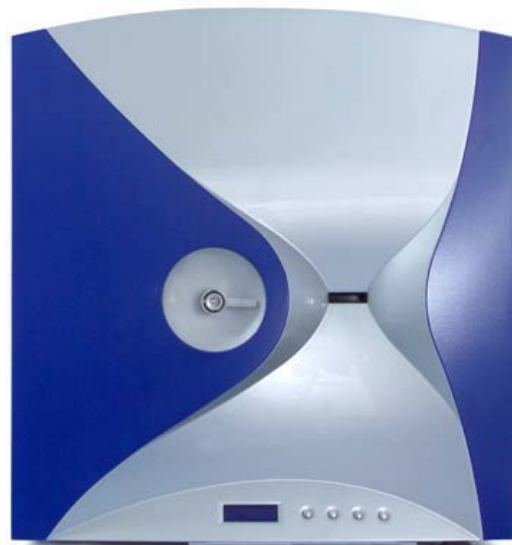
Fig 1: GENIOM – the benchtop microarray facility.
