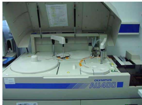
Fig 1: Equipment of the clinical chemical screen at the GMC: The Olympus AU400 autoanalyzer.
