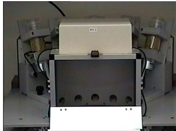
Fig 3: Five-hole box, apparatus for food-rewarded operant procedures in mice.
