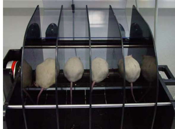
Fig 1: Rotarod apparatus for the assessment of motor coordination and balance.
