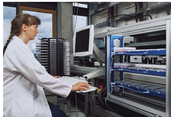
Fig 2: Liquid handling robotics used for the amplification of DNA-chip probes ensures reproducible quality and efficient throughput.
