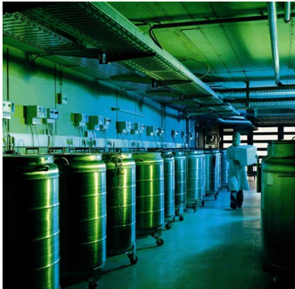
Fig 2: Liquid nitrogen tanks for cryopreservation
