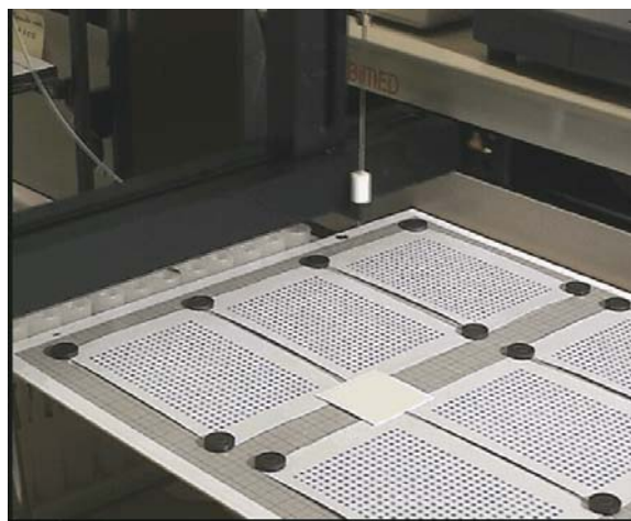
Fig 2: Parallel miniaturized chemical synthesis of compound libraries on membrane supports by the SPOT method.
